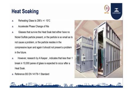
So, what to do in case of elimination of this, so that is where we are coming to our topic heat soaking. So, heat soaking is process it is a destructive process by which you reheat the glass in a oven. Here, you can see we have put the glass inside and reheat the glass into the oven at 292 plus or minus 10 degree Celsius. We accelerate the change of phase of nickel sulfide.
