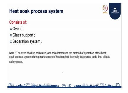
The heat process heat soak oven normally comments 3 things. One is oven for which we have a heaters, the second is a glass support, third is the separation system. The oven should be calibrated or shall be calibrated with this determines the amount at which the operation of the heat soak. The total processes depends on the calibration of the heat soaking.
