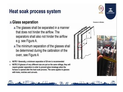
So, third part of it is the glass separator. You can see this is separators which are used. So, the aim is to have 20 mm evenly distributed over glass for example you have to have each glass the glass has to have a difference of 20 mm. And the distance of every 40 mm we need to have a separator. So, this all defined in this standards the where you have to create this spacer, how much is the space between the glass. And we normally recommend 20 mm is the space between the 2 glasses.
