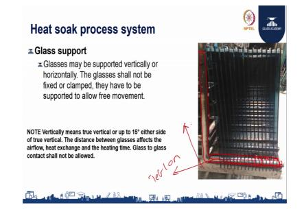
The second surface is the glass support. Now, glass support here we are talking is about the vertical or the horizontal support. So, you can see the vertical support is and horizontal support is laid such a way that the glass should not be overly having additional stress in (Refer Time: 07:47). It is normally 15 degrees inclination in max of max 15 degree of inclination is allowed. And the glass has to be separated in such a way that it is supported uniformly.
