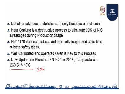
So, we are coming to end of this session. So, now couple of things have summarizes before I close. One is not all breaks post installation is because of only inclusions. Second thing is heat soaking is a destructive process which eliminate 99 percent of nickel sulfide breakages during production stage itself. EN 14179 is a standard which specifying the heat soaking and it will very detailed. And well calibrated and operated oven is the key to success of this process.
