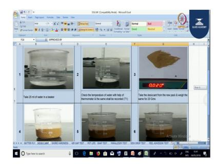
Next to test what we do is a desiccant test that we use inside the space it will absorb the moisture. If you see here the first what we do is we will be taking a 20 ml of water in a beaker. Next we will be measuring the temperature of the water then we will be taking a 20 grams of desiccants and we will be pouring the desiccants inside the water. And we will be checking the temperature after the desiccants is kept inside the water.
