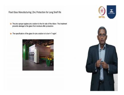
And now the glasses cooled to a temperature of a 60 degree centigrade. Now, it is time to meet the customers requirement in terms of meeting the dimensions as well as the other quality, for the glass to remain longer in a humid conditions even, to avoid the problem of weathering attack, the glass is sprayed with zinc citrate online.
