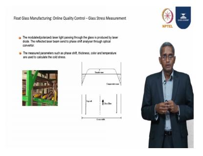
And next is we talked about the stress profile on the annealing layer, and there are online equipments which measure and tell us continuously how much is the stress on the glass, so that we can regulate and avoid bad stress glass being sent to the customer online
