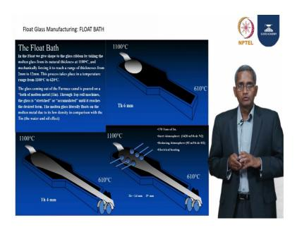
So, now having melted the glass to some extent efficiently, because we are re-generating the heat and we have now homogeneously brought the class together in the neck and we have reduced the temperature in the working end to 1100 degree centigrade, and this is a very critical temperature 1100. This is the temperature at which we can form the glass; the forming operation, like in most of the industries to work on the glass and form the glass to the shape that we want.
