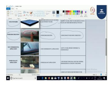
If there is a poor edge deletion you can see the traces of the coating. Our intention is the coating surface should be completely removed, and the surface should be as good as a clear glass. This is because the reason being because, of poor edge deletion and we can overcome this issue by properly doing the edge deletion and with the proper wheel to be used with proper pressure.
