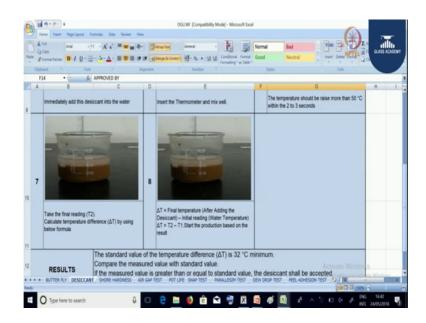
Then we will be calculating the temperature difference; that is, the temperature difference, that is after adding the desiccant what is the temperature minus initial water temperature will give me the desiccant temperature.
