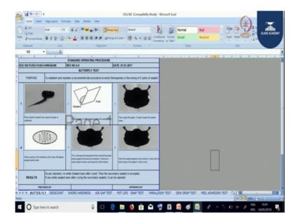
Now, let us take the insulating glass sealant. The purpose of doing butterfly test is as the sealant secondary sealant is a 2-part component. We need to maintain the homogeneity of a 2 parts of the sealant, and one of the tests which is used to see the homogeneity in the mixing is the butterfly test. The procedure what we do is, first we will be taking a piece of, we will be taking a bid of sealant onto the piece of paper, and we will be folding it
