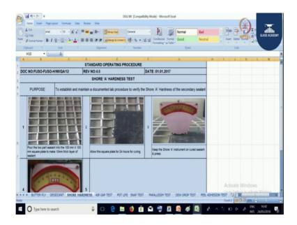
Next we will see the shore hardness test. The shore hardness test is used to check the hardness of the secondary sealant. The procedure what we do is, we will be taking a, we will be taking a 2-part sealant into a 100 mm, 100 by 100 mm square plate of 10 mm thick layer. Then we will be applying a secondary sealant on the area of 100 by 100 mm square area and after 24 hours of production we will be trying to see the hardness with
