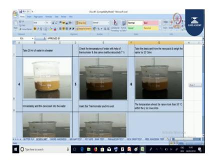
And we will be checking the temperature after the desiccants is kept inside the water. Within a fraction of seconds, the temperature will raise.
