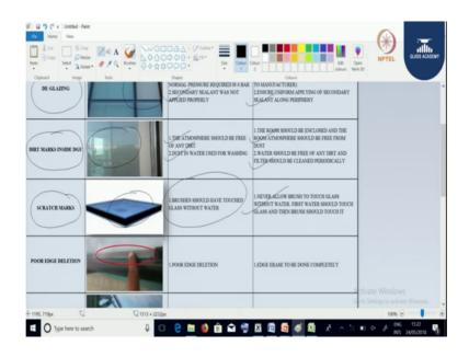
You can see dirt marks inside the DGU. You can see there is a dirt marks inside the DGU in the figure. The reason being the atmosphere should be free from any dirt and dust in water used for washing. We can overcome these issues by the room, by the room should be clean and enclosed and room atmosphere should be free from dust. Water should be free of any dirt and filter should be cleaned periodically.
