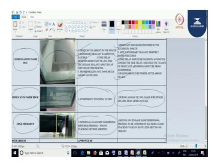
Next defect what we are going to get is the condensation inside the DGU that is, the moisture is trapped inside the DGU. The issue the reasons being, desiccant is absent in the spacer or the secondary sealant is absent in patches or time delay between the desiccant filling and the secondary sealant applying at the end of the process or proper sealing not done after organ gas is filled.
