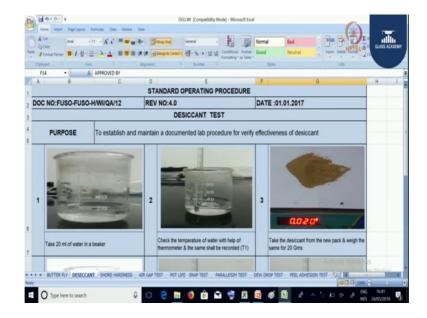
Next test what we do is a desiccant test, that we use inside the spacer to absorb the moisture. If you see here the first what we do is, we will be taking a 20 ml of water in a beaker. Next we will be measuring the temperature of the water, then we will be taking a 20 grams of desiccants and we will be pouring the desiccant inside the water.
