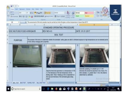
Let us take boil test. The purpose of this test is to determine whether the laminated safety glass are able to withstand exposure to high temperatures over an extended period of time without changing their properties.
