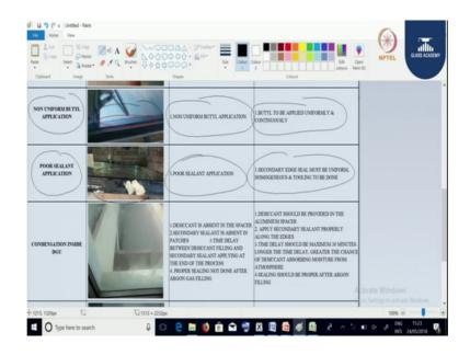
Next one is the non-uniform butyl application. You can see in the figure the butyl is like a zigzag line. Always the butyl should be straight and it should be continuous. The butyl acts as a moisture barrier. The reason being the zigzag line reason being the non-uniform butyl application, and we can overcome this issue by applying butyl uniformly and continuously.
