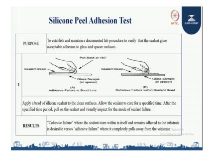
Next one is silicone peel adhesion test. The purpose of the silicone peel adhesion test is to ensure the bonding or the adhesion between the glass, silicone and the spacer. To sealant gives acceptable adhesion to the glass and the spacer surfaces. The procedure for this one is apply a bead of silicone sealant to the clean surface spacer. Allow the sealant to cure for a specified time. After the specified time period pull out the sealant and visually inspect for the mode of sealant failure.
