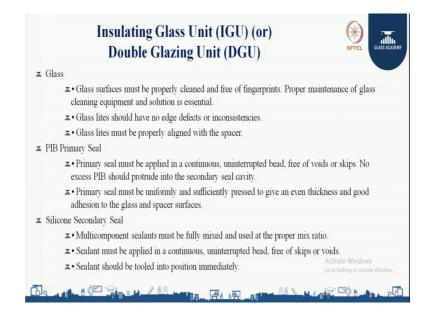
Next glass; glass surface must be properly cleaned free from fingerprints. Proper maintenance of glass cleaning equipment and solution is essential. Glass lites should have no edge defects or inconsistencies. Glass lites must be properly aligned with the spacer. Now, let us understand PIB: polyisobutylene primary seal. Primary seal must be applied in a continuous, uninterrupted bead, free of void or skips.
