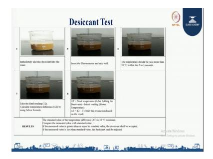
Insert the thermometer and mix well. The temperature should raise more than 50 degree centigrade within a 2 to 3 seconds. Take the final reading that is T2. Calculate the temperature difference by using below formula. The delta T is equal to final temperature after adding the desiccants minus initial reading that is water temperature. That is delta T is equal to T2 minus T1. Start the production based on the result.
