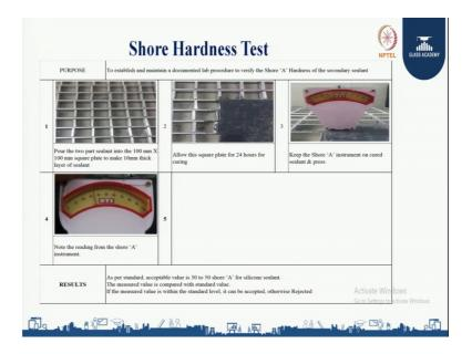
Next coming is shore hardness test. Through shore hardness test we are ensuring the hardness of the secondary sealant. The purpose of this test is to check the hardness of the secondary sealant. What we do is we will be taking pour the two part sealant into a 100 mm by 100 mm square plate to make 10 mm thick layer of sealant. Allow this square plate for 24 hours of curing.
