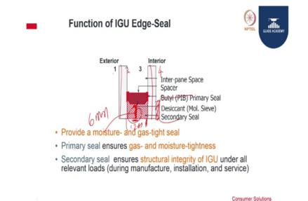
Now, we will come to the function of an IGU edge seal. So, I am going to talk about essentially the secondary seal, as well as I know how it has to be done and what other tests needs to be done while making the DGU. And I know and what are the good quality control exercise we need to do for the material as well as for the finished product.
