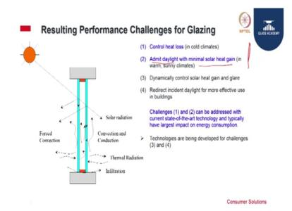
So, resulting performance challenges for glazing what do we do? We use DGU to control heat loss in cold climates these are retain the heat. So, which is exactly opposite to what we do it here and in our country like which is warm and sunny and tropical we admit daylight with minimal solar heat gain.
