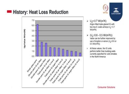
So, you know this is just to give you a brief on how the U value changes with the different composition in a DGU. So, the single glass pane will give you the highest U value it will be more conductive. So, the function of having a DGU is to reduce the thermal conductivity. So, the U value gets reduced, but you have a solar heat gain which has to be also taken care of by using a proper coating on the glass.
