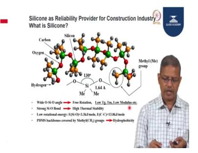
So, this is again you know explaining the structure of the material, you can see that how silicone is you know the bond angle if you really see. The silicone oxygen or the silicone by chains if you see the angle is around 130 degrees. So, this 130 degrees of angle between 2 bonds gives a excellent flexibility.
