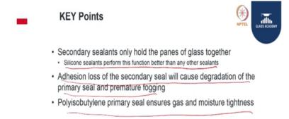
So, what is the key point? What is that we need to take away from this discussion is. Secondary sealants hold the panes of glass together. So, they are essential to structurally hold them. And silicone sealants perform this function better than any other sealants. So, we have seen n number of tests n number of experimental results, showing how silicone outperforms other materials.
