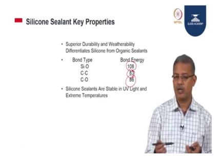
So, this let again talks about the bond energies of different materials and different chemistries. So, the first one is silicone oxygen and you can see the bond energy is 108 kilocalories ok. So, essentially if you look at so this is much higher than the UV in the sunlight energy, which is around 90 ok. So, if you look at carbon or carbon oxygen they are all much lower than the UV in the sunlight energy and that gets degraded so with time.
