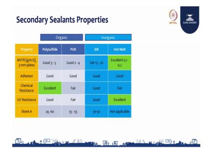
So, in polysulphide if you take it as a organic as a polysulphide, a polysulphide has excellent chemical resistance, adhesion good for all the organic inorganic and shore hardness is almost all the organic inorganic silicone. So, satisfies. So, this is the secondary silicone properties.
