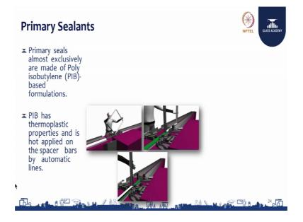
Let us discuss about the primary silicone primary seals like silicones are used extensively like exclusive are made of poly isobutylene which is mean PIB which is called polyisobutylene based on formulations it is made it. And, PIB polyisobutylene has a thermoplastic and properties it can be applied on hot applied through this spacer bars by automatic lines with the butyl extrusion machine it will be widely used for dispensing this primary silicone.
