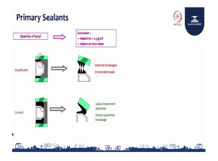
And, in quantity of a butyl extrusion like if anything is there adjust to 2.5 grams per milli and adjusted in two sides like you can adjust it. So, you can see here this is the insufficient. So, there is you know lack of you can see there is a red colour identify, there is a lack of a silicone primary silicone has been filled with it. So, will be a loss.
