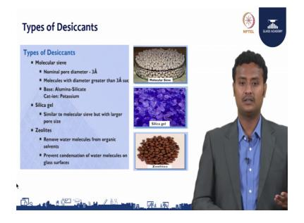
Next we will discuss about types of desiccant. This is the molecular sieve which is widely used, this is silica gel the same as good as molecular sieve, but this is the because of the pore sizes are larger in size. So, nowadays people not using it, mean it is it was obsolete not presently also it is obsolete, there is no availability of silica gel right now. And, zeolite it was once upon time was used this also kind of desiccant again this also obsolete.
