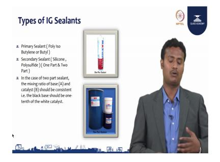
Let us move on to this type of IGU sealant. This is a single part; this is a two part silicone. So, basically primary silicone which is PIB polyisobutylene which is a single part which is primary silicone next is a double side I mean two parts which is silicone or hot melt. So, it will be a two part silicone. So, primary sealant is a PIB which is the polyisobutylene or butyl it is called and secondary sealant is silicone or poly sulphide it is like one part and two part components.
