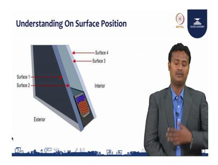
Before we get into that let us understand first the surface of IGU unit which is what site the coating portion, what glass it is, let us see about it. So, if you look at the pan like IGU unit so, you will have to differentiate with the exterior, interior which is the first most point which you have to look at it.
