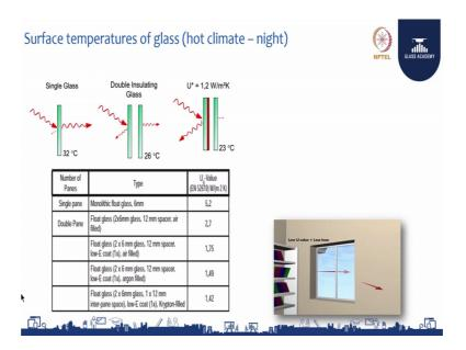
You see that single glass solar energy comes in the partly absorbed and partly reflected and again there will be a transmission in the inside the building the energy. If I use single glass I may have get it the 30 degree inside, if I use double glazed in the same thickness only there are 2 panels have increased I mean 2 panels are used it with the separation of a 12 mm then I will be getting a 26 degree inside.
