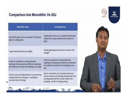
So, let us go to the main comparison between the what is monolithic glass? And what is IGU unit? So, monolithic glass is nothing but either it is annealed glass or it is a tempered glass or it is a single glass basically. Whereas, IGU glass which means it comprised our it consists of 2 or more panels together with separated with help of aluminium spacer and hermetically sealed with help of primary and secondary silicon.
