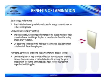
Now, coming to other benefits that a laminated glass can provide is basically Solar Energy Performance. The PVB helps reduce the solar energy transmittance. And thereby, reducing the loads onto the air conditioning and can also help you in know reducing your energy consumption that you have in the form of AC, air conditioning that you have in
