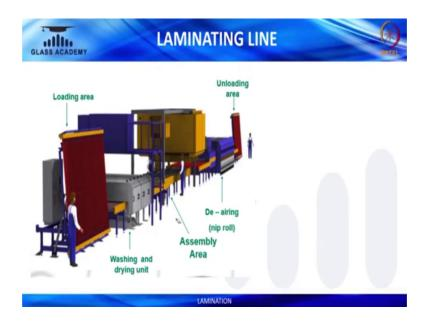
This is how an laminating architectural laminating line is designed. We have loading area, where you load the raw glass. Then, it is subjected to surface preparation, where basically we are trying to prepare a glass surface which is would be subjected to lamination in the next process. So, what we do basically is we have a de-mineralised water, we clean the glass surface using a demineralised water of conductivity less than 20.
