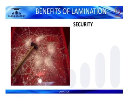
We will have a video. You can see that even after striking six times on a laminated glass using an hammer, it is not possible to penetrate through. This is what shows the vandal resistant performance of a laminated glass. That is how we call it laminated glass as part of a security glass.
