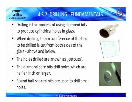
Let us start from the drilling-fundamentals. So, what is actually, if you see in the right side, there is a one picture, which is show you the drill coated on the inch or half inch of the, this cylindrical drill bits. When drilling, the circumference of the hole is to be from the both side. When you have gone to the processing line, if you see the while, who is doing the drilling, it is always should be from top side and bottom side. We also known
