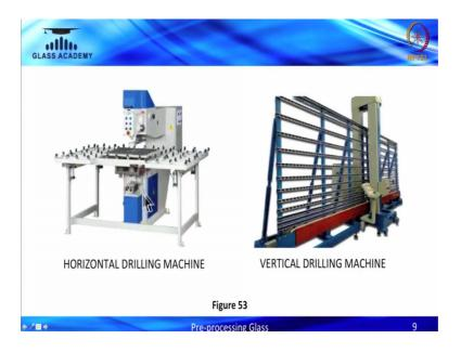
So, my next slide will be upc. This are the horizontal machines, horizontal drilling machine. And this are the vertical drilling machines. So, as I told you, it is depend upon the processor those having its facility though both have, their own advantages the comparison, I already shown to you.
