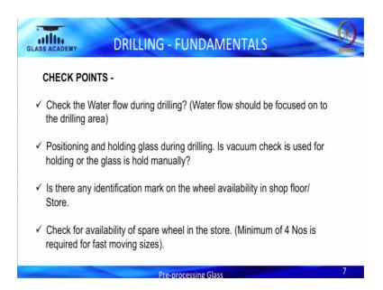
So, the next slide is what is important, when you making the drills in the holes. So, check list are there. So, you should check the water flow. So, if water will not flow properly, it mean that it will not be focus on the drill bit and as well as on the glass. So, heat will generate. So, it is very important, who is operator, who has to check. Whether of the water flow quantity or flow it is there or not.
