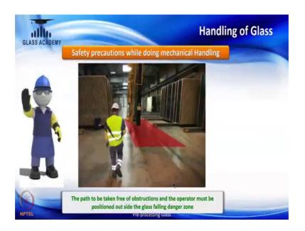
When we do the mechanical handling, the EOT crane what you can really see is the path in which you take the glass. It should be free of obstructions and operator must be positioned outside the glass falling danger zone always.
