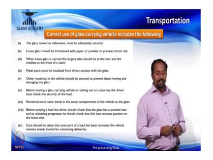
Correct use of glass carrying vehicle includes the following. The glass boxed or otherwise must be adequately secured. This we discussed and then, loose glass should be interleaved with paper or powder to prevent transit rub, then when the loose glass is carried, the largest size should be at the rear and the smallest at the front of the stack, then metal parts must be insulated from direct contact with glass otherwise glass can easily break.
