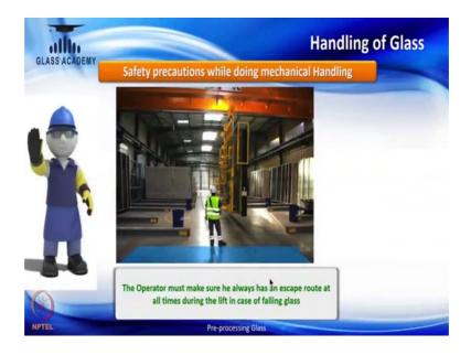
Another precaution what we need to take is the operator must make sure that he has an escape route at all times during the lift in case of falling glass.
