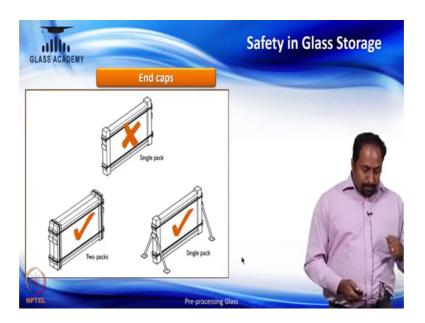
We can see the end caps here in the picture. You can see a single pack which will be very you know based on the stability what you can see single pack will not be that much stable. Then, when it is kept to stab 2 packs and then, bundled with the steel strap and all, it is safe or else you have to if you are keeping a single strap, then it has to be with the support thing, but it is shown in this picture.
