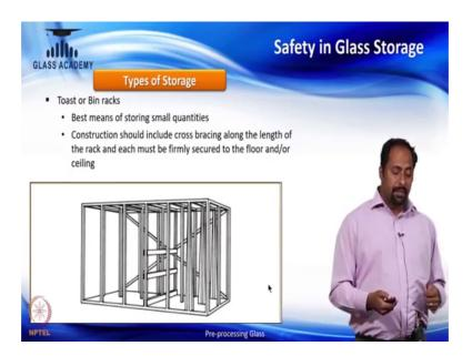
Now, another types of you know storage is like toast or bin racks. This means storing small quantities is the best one and construction should include toast bracing along the length of the rack and each must be firmly secured to the floor or to the ceiling. So, this is the way in the picture it is very clear. So, this is the way small quantities of glass what we can store.
