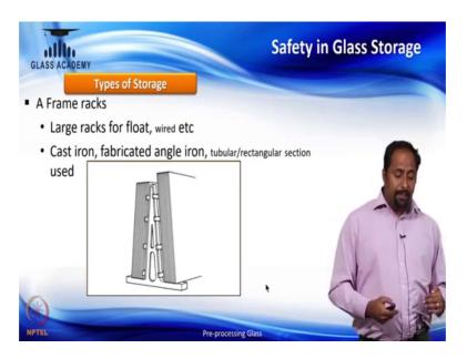
There is something called as a frame which is also very common in storage as well as transportation. So, it is kind of it has got a shape of a naive frame and with the cast iron or fabricated angle iron, then both the sides we can store the glass.
