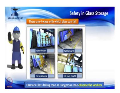
Now, that glass is stored, there are four ways with which a glass can fall and then, create an unsafe condition. So, in the first picture, what you can see is it fall sideways and another picture you can see the person how he is standing and the glass can fall on to him. So, that is fall forward and he is very much in the glass falling zone and there is
