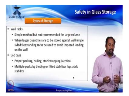
Now, what are the different types of storages? What is available as a common accepted practice? Basically wall rack system is one common method. It is a simple method and not recommended for a large volume, but when larger quantities have to be stored against wall, single sided freestanding racks to be used to avoid imposed loading on the
