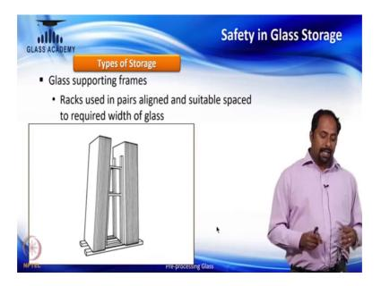
Then, glass supporting on frame. So, this is a way of we know racks used in pairs aligned and suitably spaced and based on the required width of the glass, it is very clear in the
