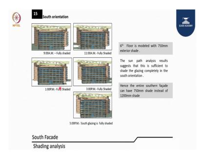
And you can look at the South orientation here we gone for little more about initially projected 1200 we optimise to 750. With the sun path analysis you can really do this kind of study and see how much is the depth required for a particular of a facade. Here up to you can see almost entire day from 9, 11, 1 pm, 3 pm up to 5 it is all fully shaded in the South.
