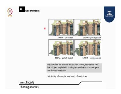
And West orientation a it is similar to East here you can see the exposed and the areas. Yes, you have a self shading and up to 2 pm you can say fully shaded. These are all shaded you can see this glass and moment is good after 3 you can see the sunlight is directly coming and hitting and after 5 we can see almost it is getting exposed.
