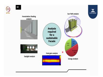
Basically, we have to go for the facade shading analysis. How that day entire 24 hours you can check for every day of the year. How the shading and sunlight fenestration to the building then daylight analysis, how this facade is giving a daylight to the interior environment where in you can control the artificial light and save energy.
