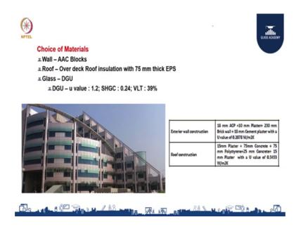
And as I told you we had all the luxury, so, we used DGU use I think they belong to the (Refer Time: 23:00) series from Saint Gobain which had 0.24 SHGC and a visual light transmittance of 39 percent and roof over deck insulation was used. So, they used 75 mm thick extruded polystyrene and for wall there was a lot of wall area.
