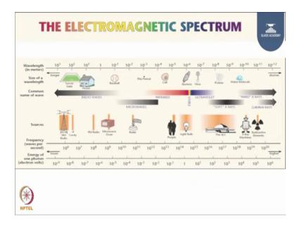
The second important design parameter I like to speak about is the UV and before we talk about UV, I am sure you are aware about the electromagnetic spectrum. And, in the electromagnetic spectrum, the one which is most important for us to discuss here today is between the ultraviolet and the infrared.
