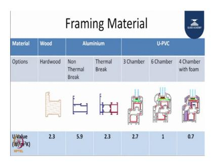
So, to give you an example about framing material for example, if you take a note you have a U-value of 2.3. You take an aluminium system and will have around 6 or non thermal break or if it is a thermal break it may have almost same like the hardwood which is 2.3. A 3 chamber PVC might be around 2.7. However, if you go for 4 5 6 4 chamber with foam you can go below 1 as well. So, a very very low U-value can be achieved in PVC system with the various configuration of multi chamber and foam
