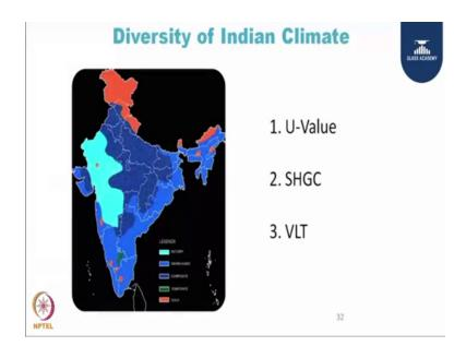
The third criteria we are going to discuss about the climatic conditions. So, India is basically divided into 5 climatic zones and based on this climatic zones one needs to have a certain parameter, which needs to be meet like U-Value, SHGC, VLT. These 3 parameters needs to be basically looked from the perspective of these 5 zones and it is specified in the green building documents from either IGBC or GRIHA.
