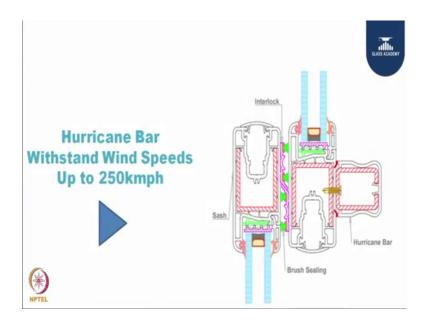
Just to demonstrate you how we achieve this strengths, this is a typical cross section of a sliding system. And, if you can see here that the red has section is the steel member which is supported with the hurricane bar. And, I will play this video just to demonstrate you how this some of these are really working in the industry so far.
