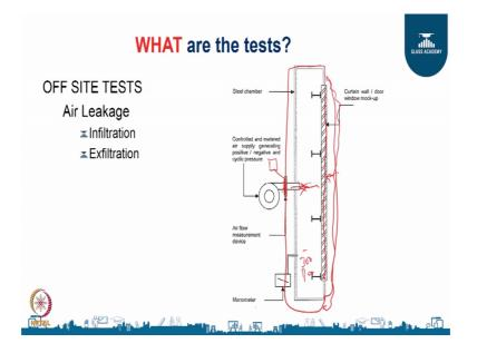
Now, what are the tests basically there are 3 tests. The first one is air leakage, and façade again is not like you know single huge piece of glass. There are thousand glasses, or 5,000 glass panels; which are coming in a series, vertically and horizontally, they are being installed at the site, and there are thousands of joints. All these joints are getting locked into each other by gaskets.
