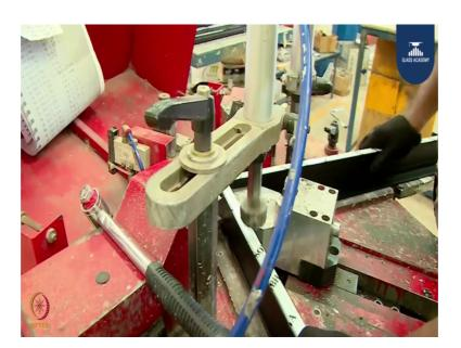
The particular section will have its own corner profile. So, corner profile is inserted from both side a crimping is done so, that this corner is attached firmly. So, here there will not be any visible member screws or anything. So, aesthetically it will be placing. There is a hidden corner cleat, that cleat will have its location for the pressing the aluminium metal.
