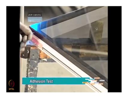
An adhesion test the post cure test is performed on 10 percent of glazing units, the test consists of cutting approximately 10 centimeters of the join lengthwise and then the sealant is pulled at a 90 degree angle to the frame. This test examines the adhesion of the silicone, its elasticity, the presence of bubbles the dimensions of the join and the cure of the sealant. If the joint is not completely cured the frame cannot be installed.
