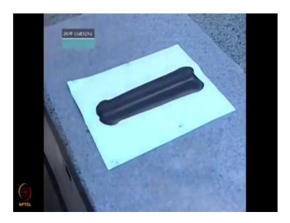
A bead of sealant of at least 15 centimeters is applied to a sheet of white paper; which is folded in half and squeezed until the sealant spreads when the sheet is pulled open again the stain must be even in colour
