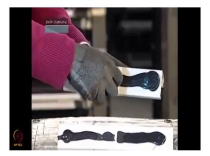
Lay down a strip of masking tape transversally, and then put down a bead of sealant approximately 20 centimetres long, making sure it passes over the tape. After the sealant has cured pull the tape perpendicular to the substrate to see whether there is any adhesive failure. If the bead of sealant does not show adhesion to the substrate the batch must be rejected; this test is to be performed at the end of each production batch.
