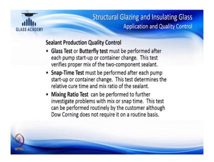
So, this can be checked by doing the adhesion testing and also the nature of failure for sealant bonding is always cohesive. So, a layer of silicone should be always stuck to the substrate, it should not come out clean like a tape or a gasket or a dry fixed system, but which does not leave any trace whereas, silicone mechanically or chemically bonds to the substrate, and then you know when you pull it tears within itself and does not leave the subject which is called as a good bonding.
