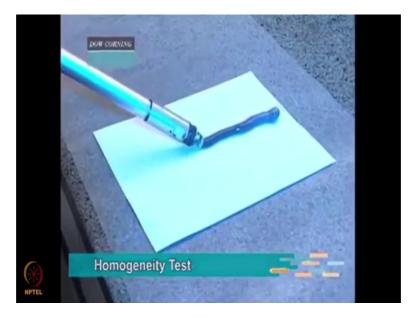
Three types of tests are carried out before bonding if a two part silicone is to be used the first is a mixing test known as a butterfly test.
