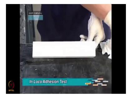
If the time observed is greater than 45 minutes, the application must be suspended. Then there is the adhesion test, clean the surface of a sample of the aluminum to be used in the project with the solvent indicated in the report and apply the primer if specified.
