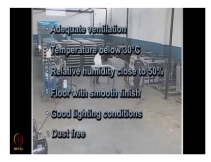
The location where structural glazing is to be performed must be reserved for the application of silicone.
