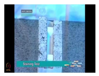
This test takes 4 weeks to complete; once the samples have been received for industry standards. If natural stone is used in the project, Dow Corning may test and evaluate the performance of its sealants to determine whether the sealant fluent can migrate into these substrates.
