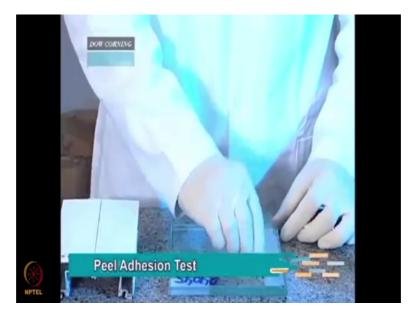
The samples must be sent directly to the laboratory after being registered in COOL. Dow Corning evaluates the adhesion of the sealants using a peel adhesion test.
