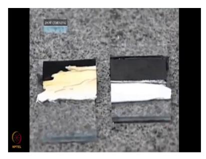
Chemically incompatible glazing accessories may cause discoloration of the sealant and or loss of adhesion to the substrate.
