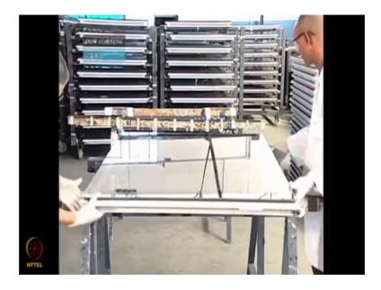
To begin the process of applying structural sealant, the first step is to clean the aluminum frame with the solvent indicated in the laboratory test result report. Using a two cloth cleaning method, if a primer is needed apply after cleaning, but primer must be applied evenly and sparingly covering the entire perimeter of the substrate and you must wait 30 minutes for the surface to be ready for sealant application.
