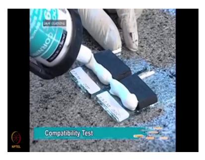
The test takes three weeks to complete, once the samples have been received for industry standards.
