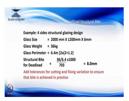
And, an example to talk about is if you have a same glass size with the 6 millimeter thick where the weight is 36 kg and if you apply the you know. So, you have a perimeter of 6.4 meters, and also you have a 36 kg. And, when you do the calculations you are getting 8
