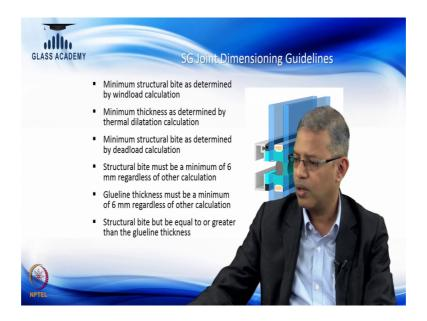
Just to recap on our first part. So, the minimum structural bite has to be always to domain by the windload, also the thickness has to be determined by doing the thermal dilatation calculations. If there is a deadload which is acting on the silicone we need to determine the deadload as per the formula. And, minimum 6 millimeter of bite has to be maintained in spite of calculations and also a minimum thickness of 6 millimeter is made to be maintained regardless of any calculations.
