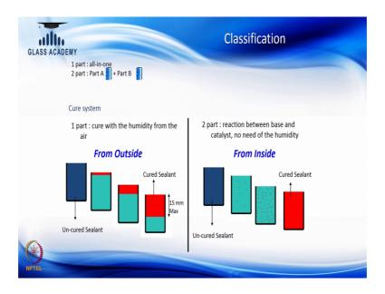
So, this sealant is converted in 2 different classified products. So, one is called as 1 part and other is called as 2 part. So, the 1 part is a ready mix you might have seen in the market a 300 ml cartridge or a 600 ml sausage pouch. So, that is a ready mix material.
