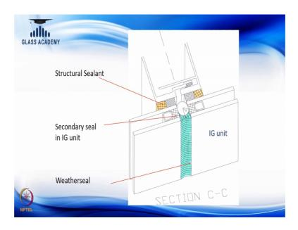
So, there are 3 types of sealants being shown in this picture; one is the structural sealant, second with the insulating glass and the weather seal. Just to give you a few you know idea. So, there are 3 products and they have different application requirement. The structural silicone is used for holding the glass to the frame and any load coming on to this unit glass has transferred through this out of the frame.
