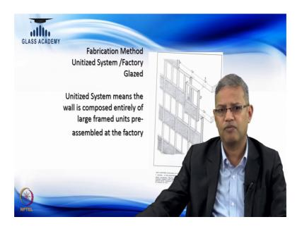
So, this is showing you the picture on the fully unitized system, you can see there is a larger frame with multiple parallels in one frame ok. It is fully unitized and this is semi unitized where in there is a single subframe. Where the glass is bonded and this is then fixed with the main frame using mechanical plates because the glass has bonded with the subframe using silicone sealants.
