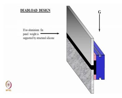
But, in some cases this may not be done this way. So, where the deadload is also taken by the sealant again this is a formula where we need to use for calculating the deadload structural bite, where the plate will act into play. So, here the weight upon you know perimeter into this is the sealant design factor for the deadload.
