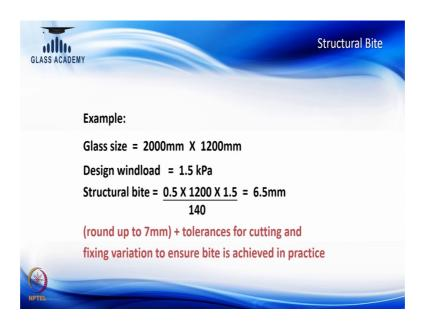
So, this needs to be calculated and this is calculated based on a formula which is again designed on a rigid plate blending theory. So, how you when you bend the rigid plate. So, what does the trapezoidal distribution of stress coming out so, based on that the formula has been developed for this technology and this is proving out to be the successful formula for last 45 years.
