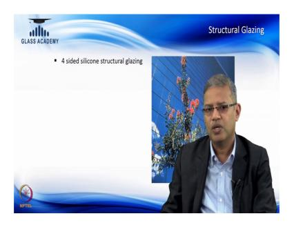
So, what is the difference you saw from the previous picture to this picture is here you do not see any mechanical fixing or an aluminium, which is holding the capping, which is holding the glass from outside. So, what does it essentially mean is all 4 sides of the glass is bonded using silicone sealant. You can get a completely clean facade by using this technology. So, you do not need to have an additional mechanical feature to hold them.
