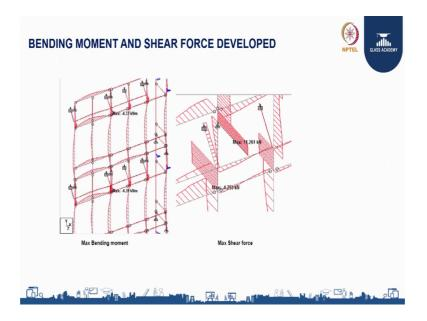
Then the bending moment and shear force has been taken from the software, that is after the application of the wind load, the dead load of the glasses and if any live load is acting on the facade.
