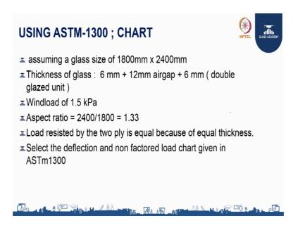
So, using the chart that is the first method and this is the second method if I will be explaining how we can determine the glass thickness or the stability of the glass using the American standard that is A S T M 1300 using the charts given in the code. Assuming the glass size as 1.8 by 2.4 meters and thickness of the glass is 612 and 6 and let us assume as a wind load of 1.5 k P a.
