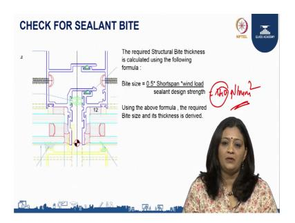
Next let us go to the Sealant Site requirement. So, the sealant bite thickness which can be calculated by using the following formula that is 0.5 times the short span into the wind load divided by sealant design strength. So, the sealant design strength is this is the standard that is 140, that is N per m m square. So, using this formula we will get the bite size required for the panel required for the panel, which is customised or which varies as per the project to project.
