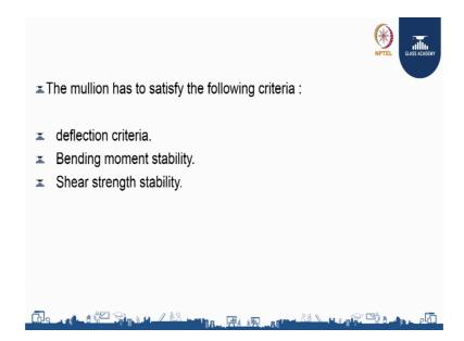
So, when it comes to the checking or the structural stability of the mullion. So, the first combined mullion will be checked for the deflection criteria and the bending moment stability and the shear force is it safe to carry the shear force. Individually both the male mullion female mullion have to be checked whether, individually whatever the load been transferred onto the mullion and that is the male mullion and the female mullion based on their distribution factors based on their inertia.
