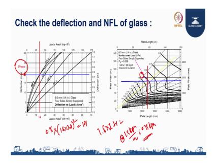
So, this is the load into area square so, where area is your glass area that is 2.4 and 1.8 that is 1.8 into 2.4. So, this will give you the area and the load shared by each glass ply that is 1.5 k p a divided by 2, which will be equal to 0.75 k P a. So, the 0.75 into your 1.8 into 2.4 whole square the value whatever you get will be 14.
