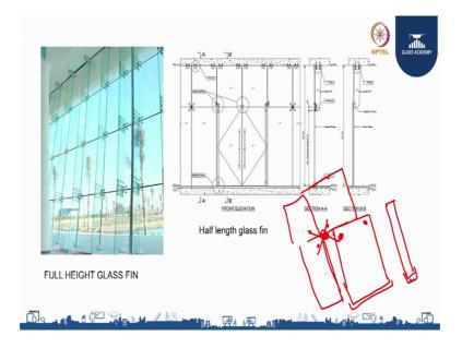
So, this shows the full height of the glass fin, this is the glass fin full height of the glass fin and this glass fin since the glass fin comes only for a span of 6 meters. So, this glass fin is connected with a splice connection. So, this in this glass fin is approximately 12 around 20 metres. So, which has two splice connection and this is the glass bottom glass, the bottom glass will be normally supported by the u channel.
