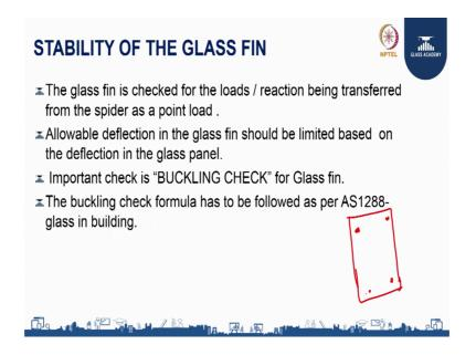
So, the stability of the glass can be used as I said in the previous methods, that is using any finite element softwares. So, in the finite element software the glass panel can be modelled like this and it with the whole and these points have to be supported and do the plate analysis. So, which gives the a result of the deflection and also the stresses developed in the glass under the wind load and also the dead load.
