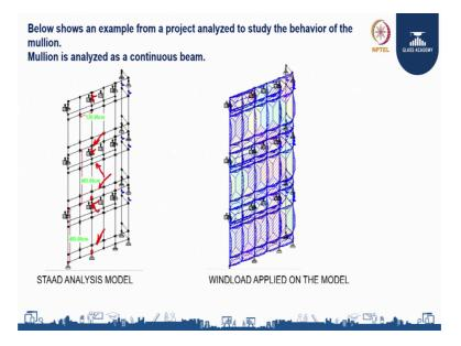
This is just a case study where in it has been where in the STAAD pro or a finite element analysis was used to analyse the stability of the mullion. Where in the panels was 1. 2 meters actually the panels was 2.4 meters we have a dummy mullion here, let us not get into that, but the panel is let us assume the panel is 1.2 metres by 4.0 metres height.
