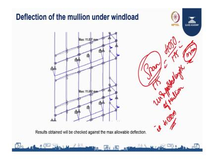
So, once all these satisfies we can always tell that the mullion is safe against the wind load or the loads being transferred, how we can derive the deflections or how we can say that the profiles, which are being used is structurally safe. So, the results have to be compared and as per I as per I S 8147, the deflection in the structural glazing or in the unitized panels is considered as span by 175 where the span indicates as the unsupported length of the mullion.
