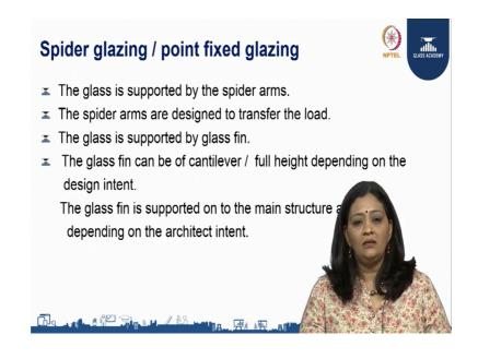
Let us go so, with the Spider glazing or the point fixed glazing. So, the glass is in this system the glass is supported by the spider arms, where the spider arms are designed to transfer the loads. So, these spider arms especially will be supplied from the suppliers or
