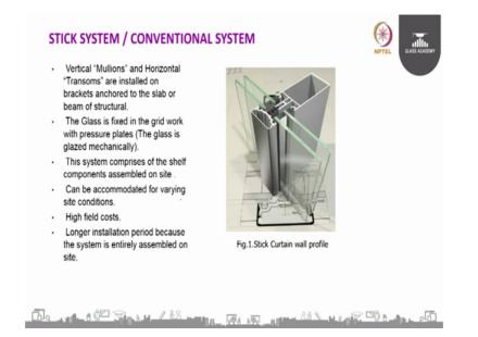
So, to brief with the stick system, in the stick system the vertical mullions and the horizontal transoms are installed and it is bind or installed and its anchored onto the slab.
