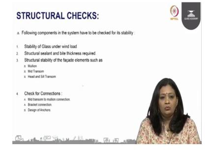
So, let us go to the structural checks mainly especially what we have to do to make sure that the facade is safe. The first check will be the stability of the glass under the wind load. The wind load is the main critical load which will be acting on the facades for which the glass is directly subjected to. So, we have to make sure that the glass panels are or the glass thickness which has been specified is structurally stable to carry the loads.
