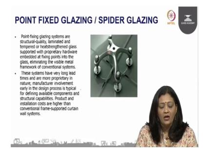
So, in the point fixed glazing the glasses the point fixed glazing or structure called laminated or tempered heat strength or heat strengthened any kind of as glasses is been fixed in the using the fixed point that is called the spiders. And these spiders are connected on to the glass films.
