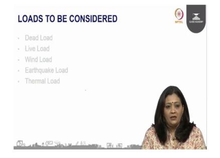
So, the loads to be considered while designing the facade; so, the first load will be the dead load which comprise of the self weight of the panels and the glass dead load these are the main dead loads which has to be considered in the design of the facade.
