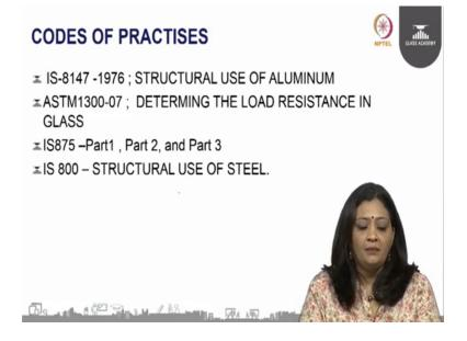
So, let us take up the codes of practices which are commonly used in the facade industry. To begin with it is the IS 8 Indian standard code of practice of a 875 part 1 part 2 part 3 which deals with the dead load live load and the wind load.
