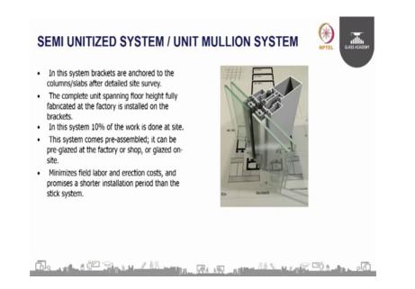
Second is the semi unitized system; in the semi unitized system so, the anchors are pre installed that is the anchors and the brackets are installed at site on the slabs or the supporting main structure.
