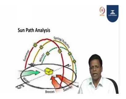
This is a simulation of sun path for the entire year for the all 4 seasons and even hour to hour. So, this will give a clarity where what are the sun penetration from the various parts of the building and elements can be designed accordingly. The ultimate aim is to have the energy efficiency in our mind and to have a complete comfort level to the occupant those who were sitting on the periphery of the building also.
