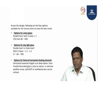
We have a very important role of selecting the vision glass where the purpose is to give sufficient light, but to make maximum insulation where I suggest a double low E glass of U value around 1 how we will achieve the U value 1. You are aware all aware that the glass single glass providing with this double low E coating may not fetch the required result.
