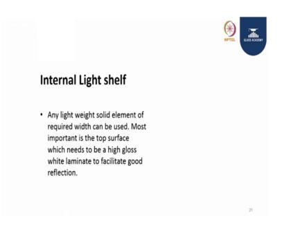
Internal light shelf of the all (Refer Time: 20:06) discussed usually will go with a MDF having top treated with highly gloss laminate bottom. We can have any laminate having of which will go with the internal interior of the building.
