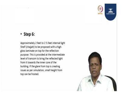
A sufficient width chajjah is proposed and a sufficiently designed internal light shelf is also designed having the purpose of cutting down the radiation and giving the light to the inner portion of the building. (Refer Slide Time: 08:28)
