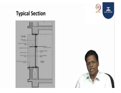
Here I am showing a typical section where this aspects of energy efficiency is kept in mind while designing the particular section. Suppose a building of 4 meter 4.2 meter floor to floor one method is to give the entire floor having facade glasses, but here in this particular section what we have what we are doing is to give around 50 to 60 percent of the glass other area we are leaving as it is for other architectural elements.
