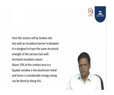
Here the aluminium sections structurally strong aluminium sections will be designed and which will be broken into two isolated from inside and outside.
