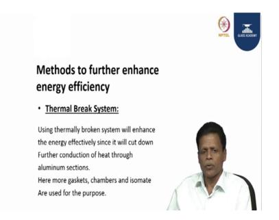
After discussing the balanced facade we have further methods to enhance the energy efficiency. We can bring down heat ingress to the building further by using this particular technique thermally broken system.
