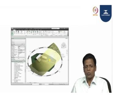
Now, one more area is suppose during the lateral movement of the sun we will have radiation even after providing sufficient width external chajjah. Here we are addressing that issue by providing vertical fins in front of our mullions.
