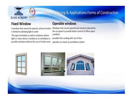
And this slide is showing various different form of window application in being a residential building or commercial building. In there are it is primarily defined by architecture and as well as a function requirement.
