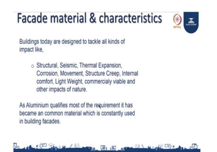
So, today a buildings are designed to tackle less we saw before. All is movement the impacts of nature commercially viable thermal expansions aluminum qualifies to all this. And any other material example you use any other metal they will become expansive one not malleable. It is very hard work with them. So, aluminum became cost effective solutions for people to consider using it façade method.
