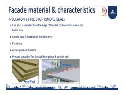
These are various examples of fire stop, how they do it is slab and then the seal it with the rock wool, mineral wool. So, this is the systems available for them you know depends on the detailing required by architect and client you design your fire stop system. (Refer Slide Time: 28:28)
