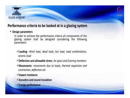
Because, it has to go through a different kinds of a test or the design requirement. Start form the loading condition which the frames are been designed for, start from the wind load or for the earthquake or for the panel dead load and the live load. So, all this has to be designed has to be considered during the design phase to define the cross section of
