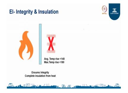
So, this is possible, because an EI glass comprises of multiple layers of glass and multiple layers of interlayer. So, during a fire, each interlayer jumps to action and absorbs all the heat as the intumescent reacts and foams up into an agent. So, if you look at the temperature values in an EI rated glass, the average temperature rise on the glass is never more than 140 degrees. And the maximum temperature rise is never more than 180 degrees.
