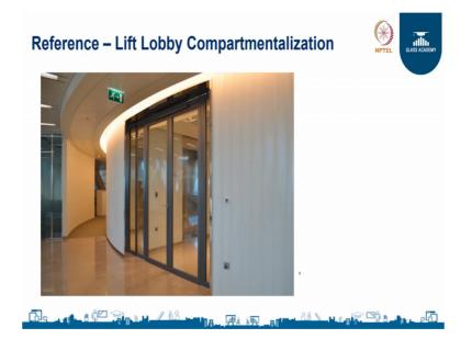
Now the advantage or the need to use a fire resistant door here is that this is the view from the other side from the area of occupancy. The need to use a fire resistant door is here is such that the fire will not spread from the main area of occupancy into the lift lobby, because there is a fire resistant door, which will prevent the fire to spread from the fireside to the protection side.
