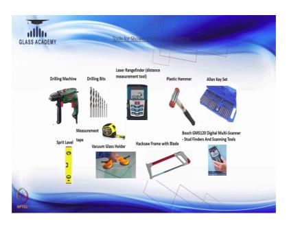
So firstly these are the tools required for installation purposes. You can see the drill machine is required, drilling bits are there, then laser measurement machine, then plastic hammering, plastic hammer sometime we need to fix the rulers and fix the plastic part into the glass. So, need not to use that wooden or iron metal hammer, you can use this rubberized hammer, then Allen key set is required.
