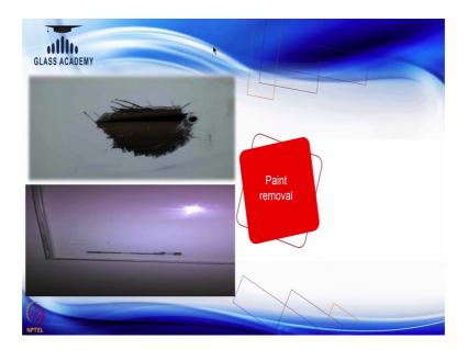
Second effects comes in this category again is a bigger picture of that defect which is known as paint removal a larger surface of that paint is being removed. Again, what the reason behind this is the same thing the incompatible issue or the improper application of that adhesive. Because of that the paint get removed from that surface causing a bad aesthetics appeal which should not be there.
