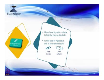
Then the second point comes in bond strength, as we discussed higher the bond strength higher the life of the glass stability. So, the recommendation here is the glass bond strength of this fixing adhesive must be of 450 kpa, because if the higher the strength it will hold the glass properly and it can hold the higher thickness of glass as well. Mostly glass in this category is used for 6 or may be 8 mm of thickness; so 450 kpa bond strength is more than enough to hold that much glass thickness.
