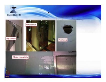
So, let us have a look on these common defects which are coming in this area because of incompatible adhesive used or improper way of application of glass fixing accessories. As, you can see the first is edge corrosion edge corrosion happening, because of the improper application of the adhesive.
