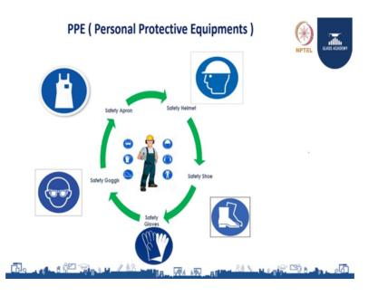
So, PPE is most important tool for glass processing industry. So, let us begin with the PPE. So, it is a Personal Protective Equipments which we all know about it. So, safety helmet, safety shoe, safety gloves, safety goggle, safety apron is most essential in terms of using the glass handling and wherever you are in the floor. So, we will have be very
