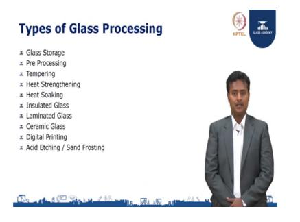
So, let us begin. So, first we are going to discuss about the type of glass processing in a processing plant. So, it is start with glass storage, pre-processing, tempering, heat strengthening, heat soak, laminated glass, ceramic glass, digital printing, basically printing, technology acid etching and sand frosting. So, these are the common typical types of glass processing happening over the world and as well as India.
