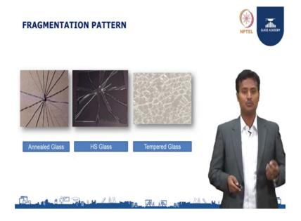
So, I would like to give you small brief about this. You see this left hand side the annealed glass breakages, you see there is lot of you know cracks when it annealed glass breaks, it is very sharp it can harm anybody and see the middle picture. So, it is a HS glass. So, typical same as good as annealed glass, but it has a strength glass with that twice than the annealed glass strength.
