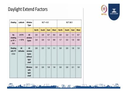
Here is a table if you look at this table carefully, it has two columns for VLT less than 0.3 and VLT greater than or equal to 0.3. Then it has two major rows, one row for no shading or projected factor less than 0.4, and the another row for shading with projection factor greater than or equal to 0.4. If you look at the first row we see that there are sub rows, one for latitudes more than equal to 15 and another for latitude less than 15 degrees north.
