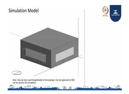
We model this in any software which is approved by the in this case we have used design builder you can see the model, it is a square building and it has window which has both the overhang and the side fins.
