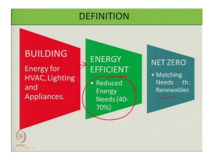
So, zero energy building net zero building or net positive building this is a concept which are coming. So, energy for building so energy for HVAC, lighting and appliances;, energy efficient, if it is next step, if you make it, you will need reduce their energy need by 40 to 70 percent, by doing a good energy efficient design. And then, matching need from renewable energy like building integrated photovoltaics you can do that can make a building net zero.
