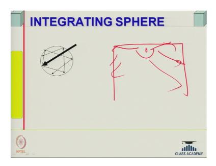
There is another principle which is used in lighting is called principle of integrating sphere. When light comes in from outside in a sphere, it will be internally reflected. For
