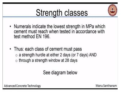
So numerals which are 32.5, 42.5 and 52.5 indicate the lowest strength in megapascals which cement must reach when tested in accordance with the test method EN 196, it is the lowest strength. It is not the characteristic strength, it is the lowest strength, in IS we call it the characteristic strength. Each class of cement must pass a strength hurdle of either 2 days or 7 days that is the early strength hurdle is 2 or 7 days.
