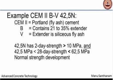
Again another example is given here CEM II B-V 42.5 N. So again it has got strength requirements, it has got compositional requirements and so on and so forth. Now in EN standards there is no performance based specification like in the ASTM standards. Now there ASTM is taken a step forward and given a very challenging scenario to the cement producers that they can actually come up with cement that match performance requirements.
