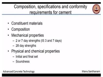
Of course there are requirements for the constituent materials, and the composition, there are requirements for the mechanical properties of the cement, as per the Euro Norms it is 2 or 7
