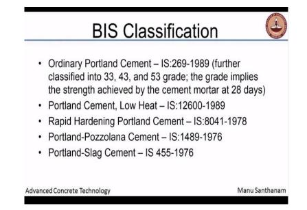
Which is further classified in terms of the strength grade. In India, we have 33, 43 and 53 grade cements, okay, and the grade implies the strength achieved by cement mortar at 28 days. So obviously at 28 days, the 33 grade cement obtains the strength of 33 megapascal plus a certain
