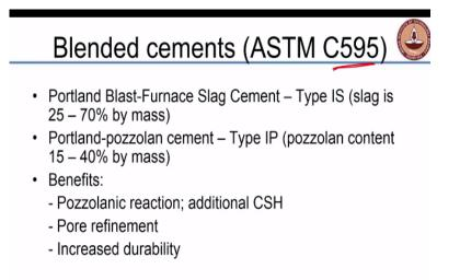
Now the blended cement, primarily there are 2 types, one is Portland Blast-Furnace Slag Cement, it is called type 1S and type 1P for pozzolanic cement or Portland-pozzolan cement which we have in India also we will call it as PPC. In India we call this a PSC of course and this is PPC. Slag content in the Portland blast-furnace slag cement is about 25-70% by mass.
