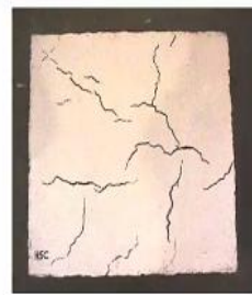
HSC, C70 Crack area = 2150 mm 2
