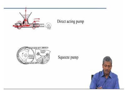
This is just diagrammatic representation and here you can see the Direct-acting pump has a piston that is trying to push the concrete. There is a hopper into which the concrete is poured from the truck,. And there is a valve which opens to ensure that the concrete continuously gets filled up into this pumped section.
