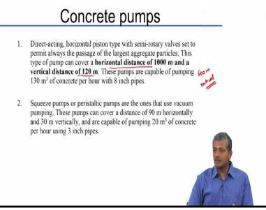
So there are different types of concrete pumps that are used in construction. There are 2 principal types of pump one is a Direct-acting piston type pump which essentially applies pressure with a piston. The other is the Squeeze pump which uses vacuum to pull the concrete. A piston pump
