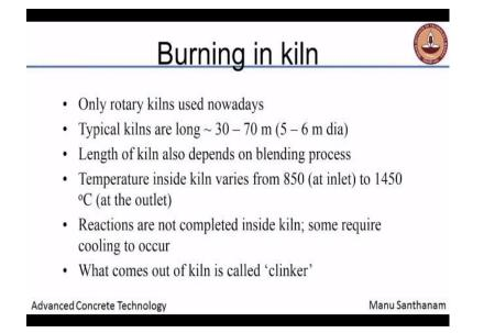
Now moving on to the most important operation in cement production, the reactions that happen in the kiln, okay. So obviously this reaction is termed as calcination, when we burn the raw materials in the kiln we call it the calcination of the raw materials and as I was telling you earlier we only use rotary kilns nowadays, we do not use vertical shaft kilns for the many advantages that rotary kilns actually give you.
