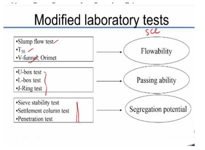
So, what we need to rely on when we deal with self-compacting concrete are empirical test methods which are modified laboratory test, which can actually give a much better picture than the regular conventional slump or workability based tests. So, the flowability for example, if you apply this to SCC, there is 3 primary characteristics that you need to measure for SCC, there is flowability, the passing ability and segregation potential.
