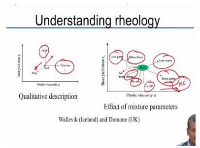
So, here plastic viscosity is depend on both parameters, so how do we understand rheology, we understand it primarily with the use of these 2 parameters; shear yield stress and plastic viscosity, so this is your reference mix for which you are able to determine through rheological experiments the shear yield stress and plastic viscosity, compared to the reference mix if you say that you are making a mix that is wet.
