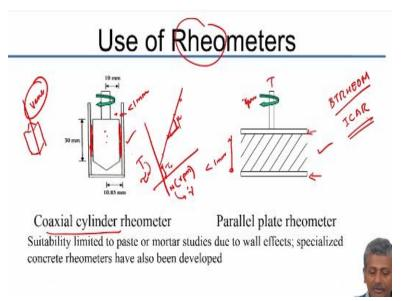
So, in terms of direct measurement of rheology views what are known as the rheometers measurement of rheology is done with rheometers, the 2 conventional geometries of rheometers is
