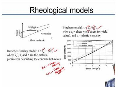
The convenient approximation we are looking at is the Bingham model where 2 unknowns are: shear yield stress and plastic viscosity and you can represent that by a linear equation:
