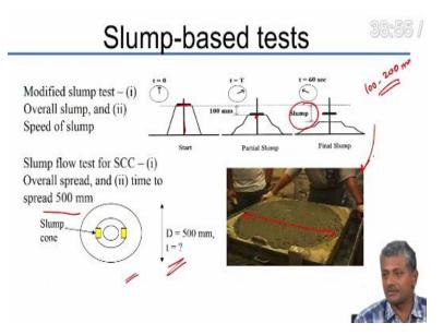
So, let us look at these test briefly, the slump based tests; the primary one which is used by SCC, looks at the slump flow which is basically the concrete which is poured inside the slump cone, you remove the slump cone very fast and allow the concrete to start flowing and you measure the total flow by measuring the diameter of the spread, you can also measure the time taken to spread 500 millimetres.
