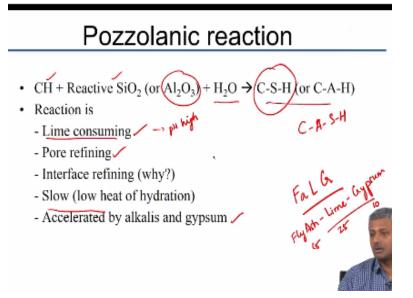
But they need the presence of lime for reaction to be completed and production of additional CSH. So, of course, just to reiterate, the Pozzolanic reaction involves calcium hydroxide with reactive silica or alumina, sometimes the Pozzolanic material may also have reactive alumina for example, we saw several types of Pozzolans like class F fly ash or metakaoline, they will also have alumina, which is quite reactive or amorphous.
