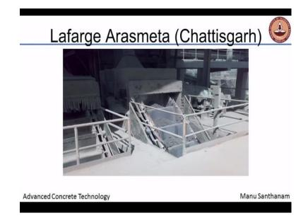
This is the clinker that is coming out of the cooler. You can see the clinker looks like a very nodular almost like an aggregate, right, and that is basically your clinker which is fused together at high temperatures and after cooling it comes out like nodules.
