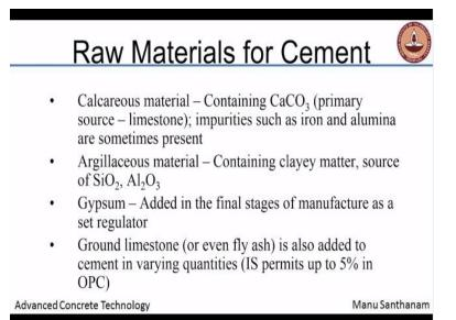
So coming to the raw materials for cement production, we know that the primary raw material is the same that was previously used for lime that is calcium carbonate. So it is essentially calcareous material, it need not be just the limestone, it could be other forms of calcium carbonate which have certain impurities also. I will talk about that in just a minute. The source of your lime may also have some impurities in the form of iron and alumina.
