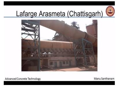
So this is the rotary kiln here. That's your rotary kiln and this is the heat recycling tube that is actually taking up the extra heat and conveying it back to the preheater tower. So the rotary kiln, please remember it is a very long cylinder nearly 40 meters in most dry process plants if not more, okay and what you also have to imagine is it is made with steel and steel cannot withstand extremely high temperatures.
