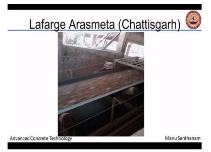
And this is the conveyor which is taking the limestone from the stacking yard towards the crushing unit.
