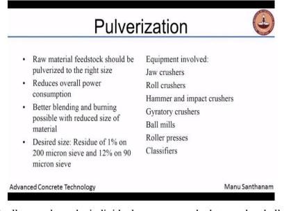
Now, we will talk now about the individual processes and what are the challenges involved in these processes. You know that the first important process is the pulverization of the raw material. The feedstock of the raw material should be pulverized to the right size, again as you rightly said for proper blending and burning of this material. So if you are reducing the size, it reduces the overall power consumption to get a certain quality of your cement.
