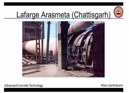
So again this is the picture from the left side so that is the preheater tower that is the rotary kiln. You can see that the slope is very gentle, the slope is extremely gentle because the material should come in at a fairly controlled speed, okay, and at this end that is at the lower end of the kiln, is the fuel source.
