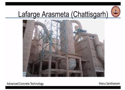
Again from the crusher, the material is stored in a temporary silo, and there will be other temporary silos for other raw materials which you want to add during this process.
