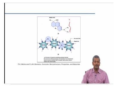
So this is a snapshot from Mehta and Monteiro book which tells you the working of airentraining chemicals. The picture in the top is the basic molecule of the air entrainer. Mostly air entrainers are derived from again tree extracts like vinsol resin.
