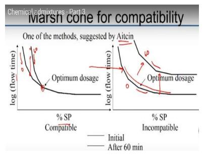
Now what Aitcin and his colleagues at Sherbrooke university have come up with is that for a compatible combination the flow curves at time=0 that means right after mixing the cement and water and at time T=60 minutes that means 60 minutes after mixing. The flow curves coincide after 60 minutes. So for a comparable combination the flow curves at 0 and 60 minutes coincide after the optimum dosage.
