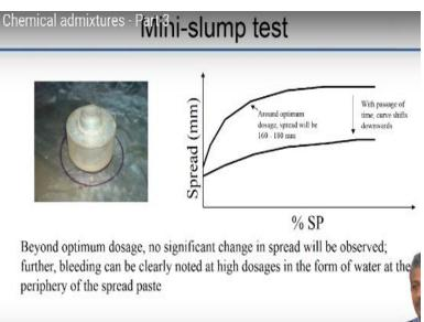
Okay there is another test which can be used and it is typically done alongside the Marsh cone test and this is called a mini slump test. As the name indicates it is actually just a miniatured version of the slump cone. So, here we are talking about an opening diameter on the top of about 20 millimeters. The diameter of the bottom which you do not see very clearly is about 40 millimeters and the height of the slump cone is 60 millimeters.
