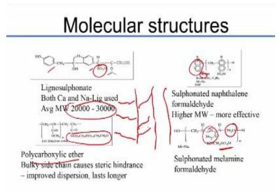
The molecular structure is defining the structure of the monomeric unit. So in lignosulphonates, you see that there are several benzene rings and then you have the sulphonate group which is attached to the long chain and in terms of the molecular weight, the average molecular weight is about 20,000 to 30,000, so higher the molecular weight, the more the effectiveness of the admixture.
