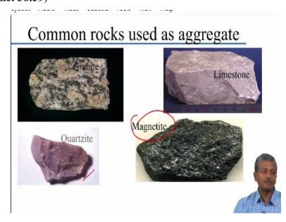
The common rocks that are used as aggregate you know very well, granite, limestone, magnetite, and quartzite, where is magnetite used as aggregate? For high density concrete because magnetite is iron; made with iron because of that it lends a very high density to the aggregate which contributes a density to the concrete and where do you need high density concrete? For nuclear radiation shielding, it is used only in nuclear reactors for radiation shielding purposes.
