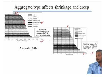
Aggregate type primarily affects dimensional stability shrinkage and creep, and these are relative shrinkages of concrete for different aggregate types, of course, the water to cement ratio of the concrete is fixed to enable comparison across a different range of aggregates, so here you see your relative shrinkage for different aggregate types and a relative creep for different aggregate types.
