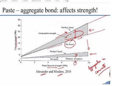
So, how does it affect concrete properties? One first and foremost property is the strength of the concrete and the paste aggregate bond has known to affect strength and people have shown this
