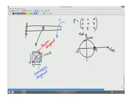
When I subject a bar, fix this in subjected to a torsional moment T ok. Now I subject this to a torsional moment the maximum shear stress occurs where maximum shear stresses in the plane of the problem ok. So, the state of stresses pure shear 0 0 0 0 0 tau, 0 tau 0 for example, and the Mohr circle for this is sigma of n taus of n shear stress it will be a circle there where this is tau this minus tau this tau max.
