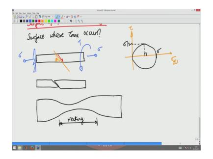
So, let us take the example of a Uniaxial tension surface of failure in the body that is we said that when tau max occurs it will fail right. Now, what we are interested is finding that surface where tau max occur. So, that will determine this our failure.
