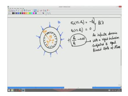
Now I can now, another boundary condition wherein the inner surface can be yield fixed say I have a rigid body a rigid steel rod put into a rubber pipe and I am pressurising this pipe from outside. Now I am pressurising this pipe from an outside pressure say from outside pressure pe what is the boundary condition now?
