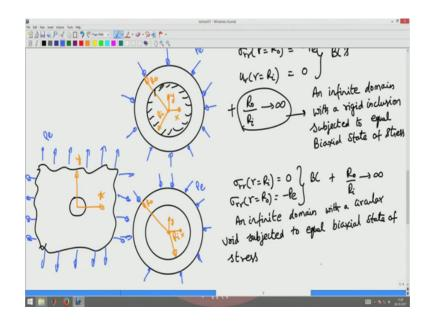
Similarly, I can have a case of an external pressure alone applied in this domain pe an external pressure alone applied in this domain wherein now the boundary conditions is obvious should be sigma rr at r equal to R i has to be equal to 0 and sigma rr at r equal to R naught would be minus pe, and for this boundary condition plus the limit R naught by R i tending to infinity, you will have an infinite domain with a circular hole in the middle subjected to an equal biaxial state of stress ok.
