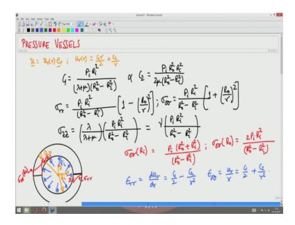
The displacement field u of r has to be given by C 1 r by 2 plus C 2 by r and then we found the constant C 1 and C 2 such that the boundary conditions for the given problem are satisfied. In particular in this problem, we are pressure appear at the inner surface and no pressure applied at the outer surface.
