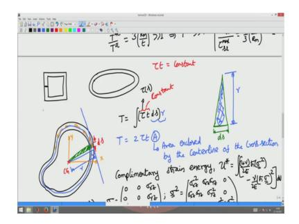
See what is the stress distribution or how is the torque and the angle of twist related, and how is the maximum shear stress and torque related for this square cross section thin walled square cross section.
