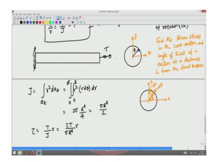
Now, I want to find what are the stresses find the in particular; I want to find the shear stress in the cross section and angle of twist of a section at a distance L from the support from the fixed support. So, this is what I am interested in finding. So, to find the shear stresses I have to first find the polar moment of inertia torsion is given as t.
