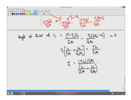
So, to twist at C angle of twist at C at C is given by T minus T C into L 1 by J 1 mu 1 minus T C by J 2 mu 2 into L 1 plus L 2 minus L 1 must be equal to 0. So, that gives you T C into L 1 by J 1 mu 1 plus L 2 by J 2 mu 2 must be equal to T into L 1 by J 1 mu 1 right ok.
