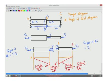
Now, let us assume that this has J 1 as a polar moment of inertia, this has a length L 1 and mu 1 is the shear modulus of this material let us assume this as having a length L 2 J 2 and mu two are the polar moment of inertia and the shear modulus of this second shaft, let us also assume that this is A B and C. I am interested in finding what is the torque diagram and angle of twist diagram I am interested in finding these two ok.
