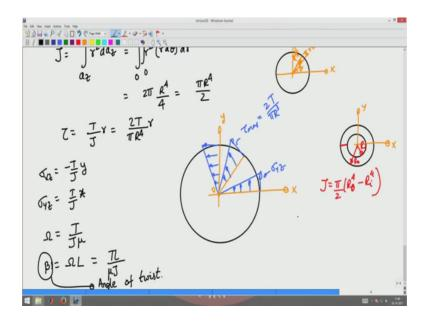
So, I have this cross section which I have zoomed out. So, the centre of the cross section is this x, this is y. I know that the shear stress is varying linearly radially which means that the centre where r is 0 here stress is 0 here and then if I look at some radial distance r I the shear stress is going to vary linearly that is going to vary something like that going to vary linearly like that.
