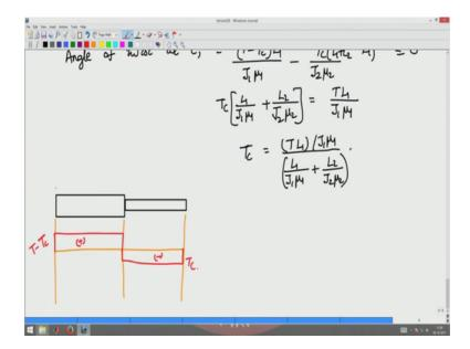
The torsion diagram would be the following the torsion diagram would be the following in this member there is a negative torsion T C is an ideal torsion T C and here there is T minus T C. So, basically this is a torsion diagram for this structure which is fixed at both the ends ok.
