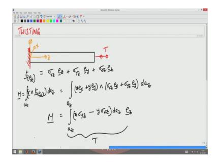
So, till now we have been using x y z over in a particular fashion, but now I will orient x y z in a different manner ok. I have this cross section and for me now z is the axis of the beam y still remains the vertical, but the x is oriented like this. So, this is the axis that I am going to use.
