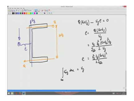
Now why do I want, I know that the channel section there is this net force Q acting like that. And net force Q acting like this and this distance this what I am interested in. That distance would be h plus tf. And there is this shear stress sigma XY which will if I integrate I will get it as Vy there Vy and I have this externally applied load acting at some distance e from here.
