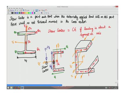
Now, let us proceed with the channel section or the C section here, how will the shear force how will the shear vary to the bending in m z direction? The shear stress is going to vary something like this. Let us make a cut here, make a cut there. If I make a cut there, and mz pass mz moment produces compressive force on the top flange. There is that compressive stress coming on the top flange, which is computed by mz by I z z into y minus y naught.
