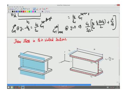
So, till now we have been looking at shear stresses in thick wall section. So, now we look at shear stress in think walled sections. So, now let us look at this I section which is thin walled subjected to some bending moment, wearing bending moment along he axis of the beam.
