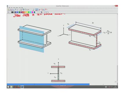
Basically there is these shear stresses arise to maintain equilibrium of the sections when there is a varying bending moment. It is not necessary that always this varying bending moment should produce only sigma x y shear stress; you can produce even sigma x z shear stress as we see here.
